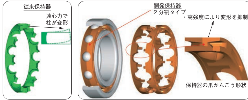
図8 高強度樹脂保持器付き深溝玉軸受 4) Ball bearing with high-strength resin cage 4)
