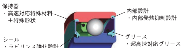
図30 電動過給機用玉軸受 Bearing for electric supercharger
