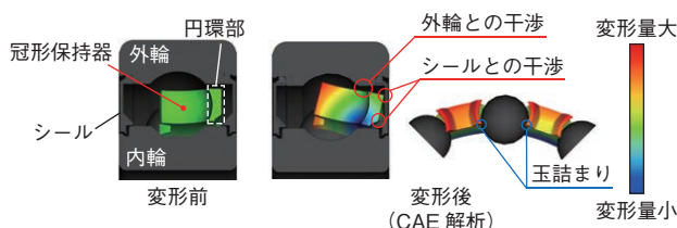
図3 変形による冠形保持器と他部品の干渉 (CAE 解析) Interference between snap cage and other parts due to deformation (by CAE analysis)
