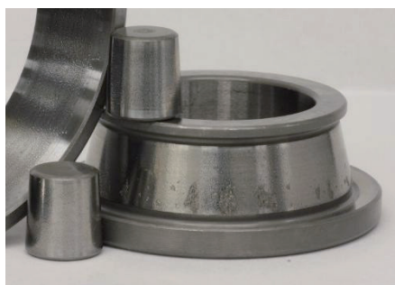
図8 圧痕起点剥離寿命 Dent-initiated spalling life
